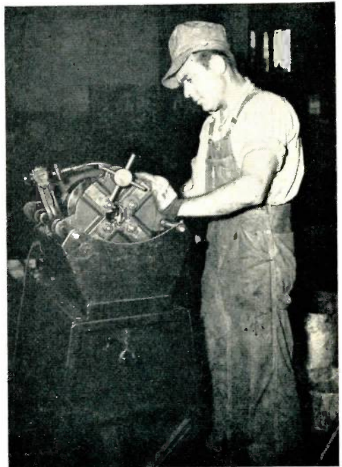
Howard Atteberry, plumber, threads a three-quarter inch pipe on a pipe-threading machine. A similar machine is used by the maintenance department's electricians to cut and thread conduits.
