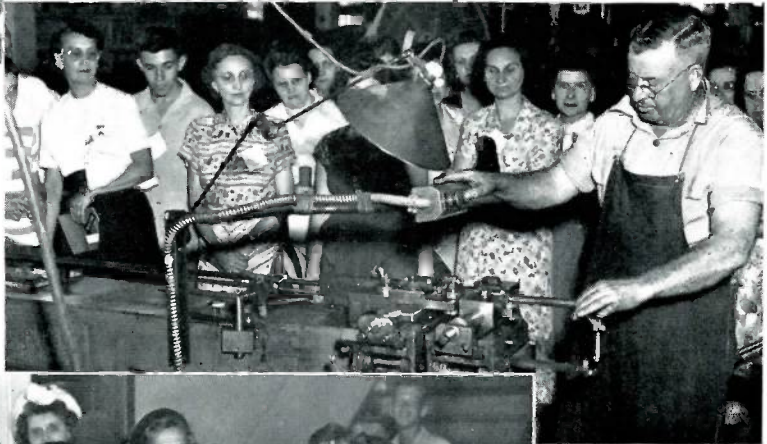
Dan Truett shows a group how copper tubing is bent to close tolerances for meter risers.
