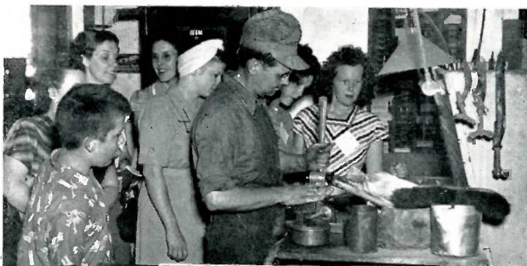
Myrle Carter, head coremaker at Plant No. 2, drew an appreciative audience as he deftly made cores for iron castings.
