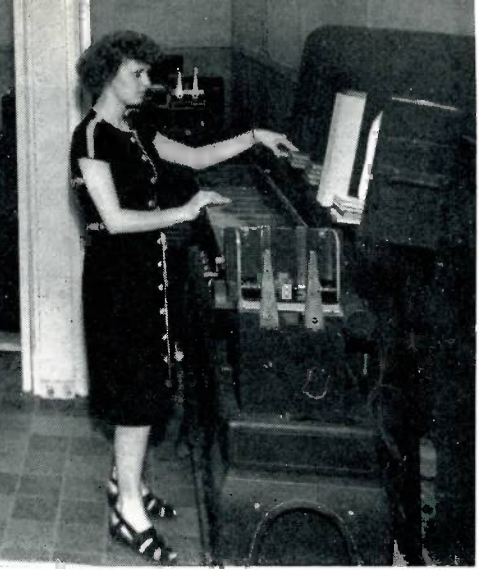
below, with a plugboard for a tabulating machine. Many combinations are possible.
