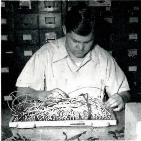
Ted Hunter, IBM customer engineer, checks tabulating machine's intricate wiring system.
