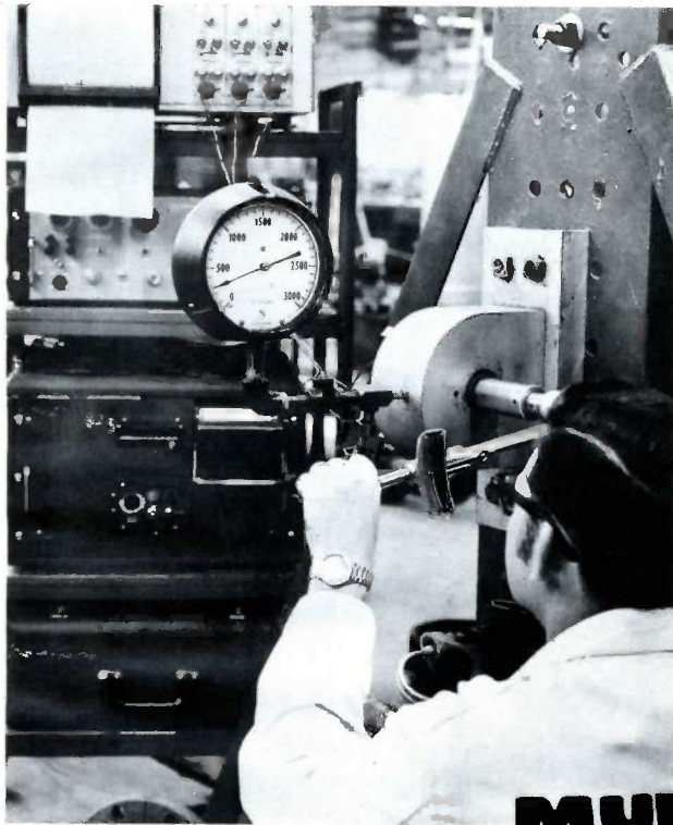
Testing of clamp bolts to determine load developed by bolts at various torque levels.
