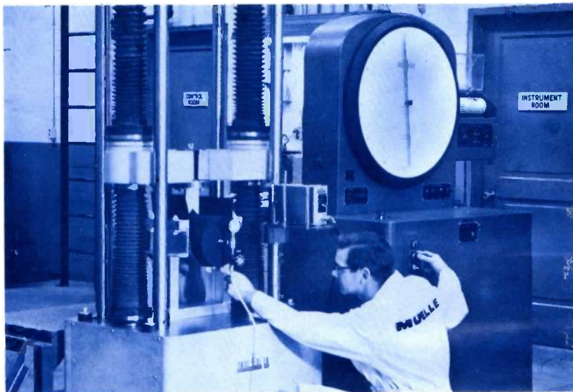
Testing gasket material and grid configuration to determine pressure sealing capability and optimum gasket loading.
