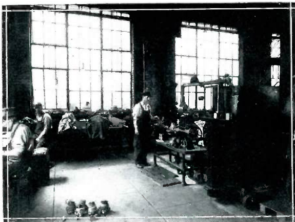
The meter testing department at Grand Rapids showing a Mueller Water Meter Tester in operation.
