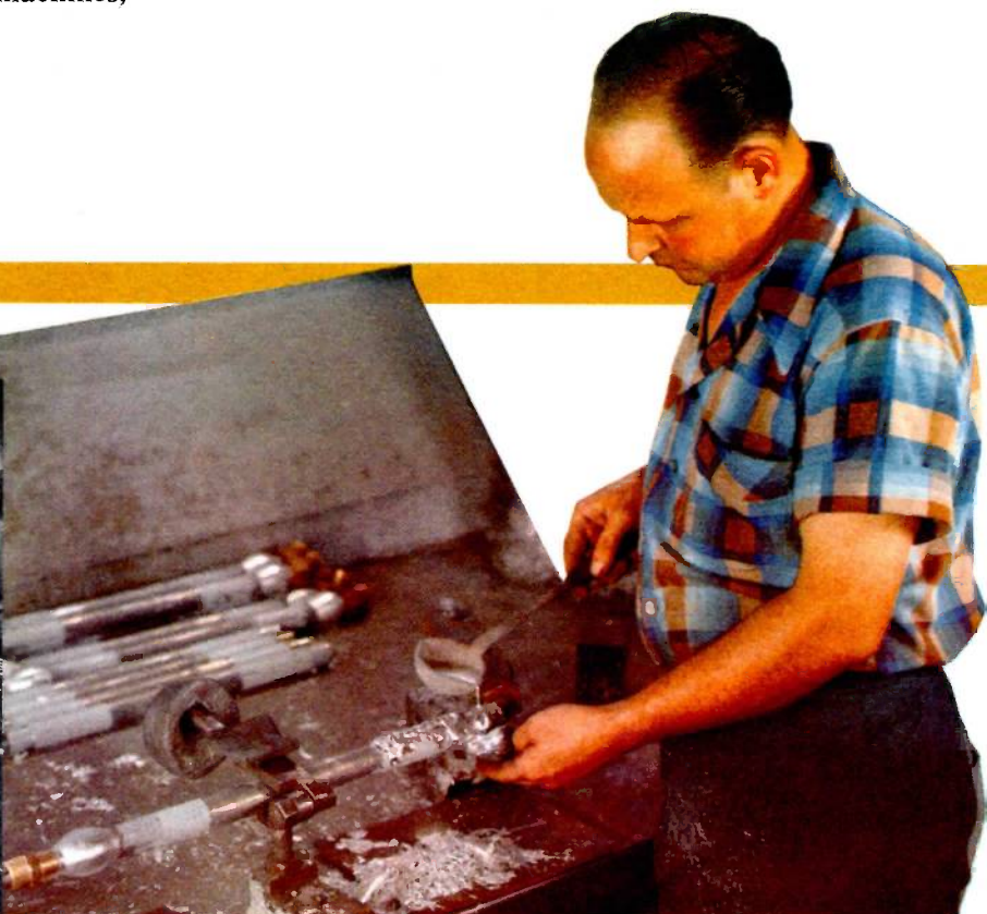
A skilled workman with a steady hand and a "fire-proof" thumb "wipes" a lead gooseneck joint to mirror-smooth perfection.
