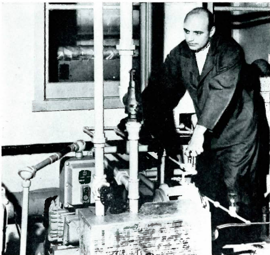
A technician adjusts dials on a sea water conversion apparatus which is part of a process that freezes sea water in order to obtain fresh water in the form of ice crystals.
