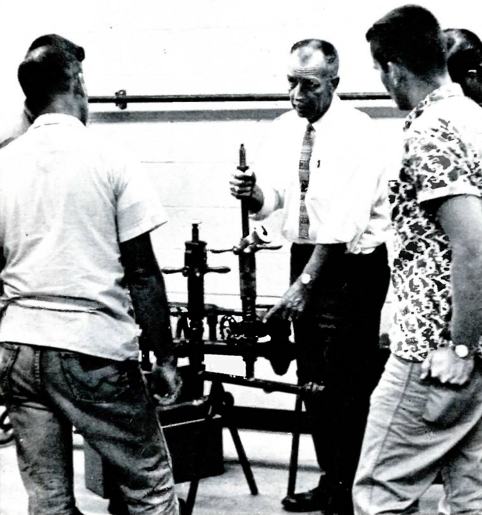
Tool Supervisor Lloyd Shannon reviews techniques for using a Mueller drilling machine for the Northwest Natural Gas Company employees who, during their training period, will make a cut on a line under pressure.
