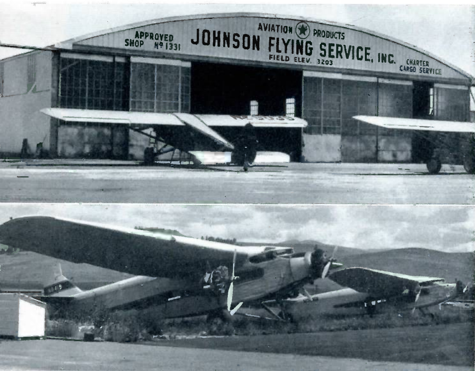
ABOVE, The Johnson Flying Service hangar. Below, two Ford tri-motor planes, the type used to drop 70 feet of water mains by parachute high in the Montana mountains.
