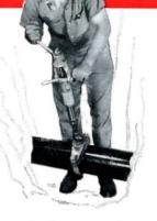
double strap service clamps provide the proper clamp and corporation stop for every application. The versatile E-4 machine permits connections to be made under pressure quickly and economically.
