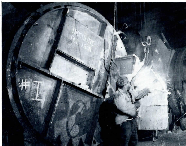
Furnace operator carefully fills ladle from one of four electric induction furnaces used to melt scrap steel and pig iron into high grade cast iron used in valves.
