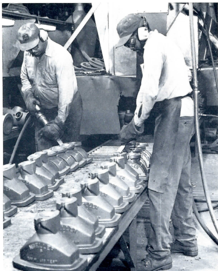
Grinders remove fins, gates and other rough spots from castings. Knowing what and how much to grind away is critical job. How well the final product looks depends largely on how well grinders do their work.
