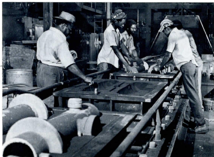
Below, molds are automatically made on this 300-foot long Mold-master. The "monster" automatically fills, rams, closes, weighs, indexes and shakes out molds.
