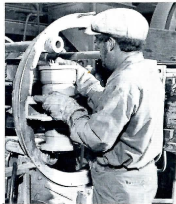
Furnace operator carefully fills ladle from one of four electric induction furnaces used to melt scrap steel and pig iron into high grade cast iron used in valves.
