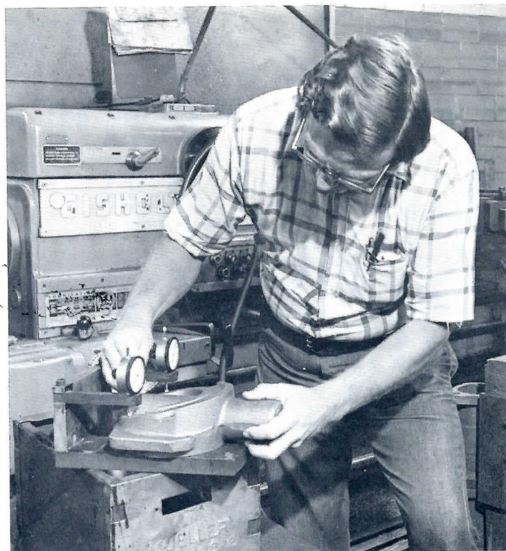
Are angles on wedge disc accurate? Dual-gauge instrument tells the inspector what he wants to know. Testing and inspection are conducted throughout manufacturing process to assure the high quality level that has always been a Mueller trademark.
