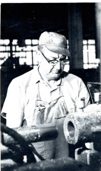
Alex Bogaart, a 30-year employee, operates a multi-spindle, semi-automatic chucker which is capable of machining either brass or iron.
