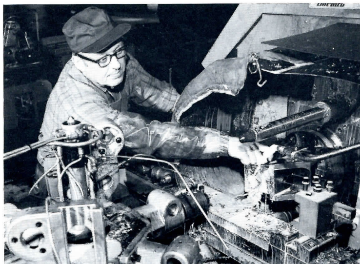
Loading a steel forging into the chuck of this machine is John Round, a 36-year employee. In this situation, the lathes are fully automatic and one man operates two machines.
