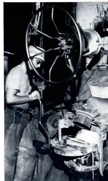
Induction furnaces are recognized as one of the cleanest and most efficient melting processes in the industry. Here, Barry Hopkins carefully fills a pouring ladle from one of a bank of three induction furnaces.
