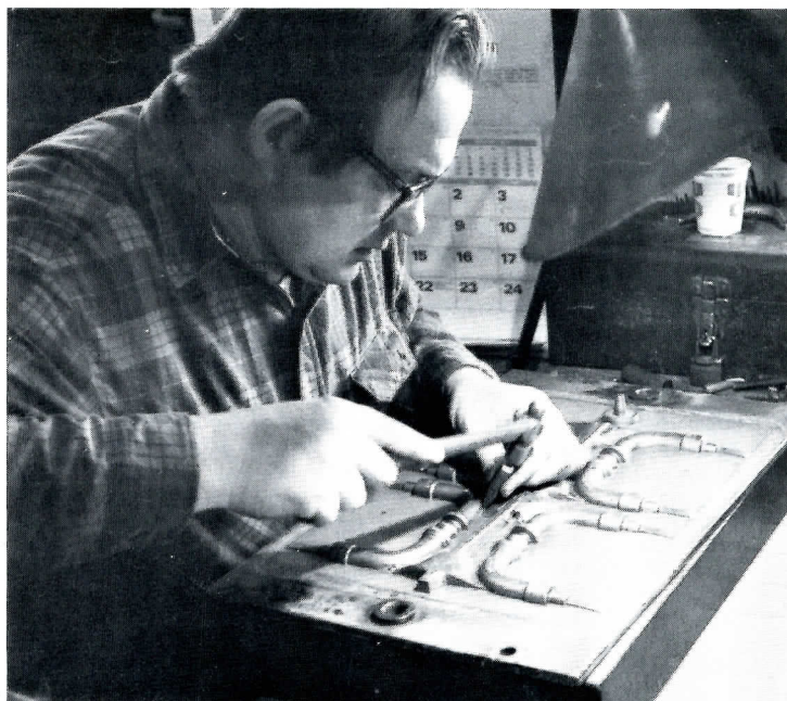
Pattern maintenance is the responsibility of the Pattern Shop. This pattern maker takes great care in repairing a pattern.
