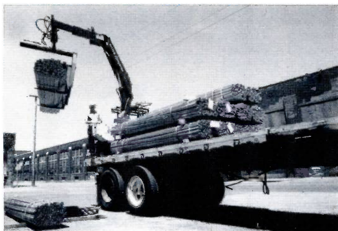
A kangaroo crane allows the driver to work unassisted.
